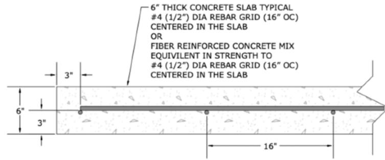
TYPICAL 6" CONCRETE SLAB DETAIL (NOT TO SCALE)
