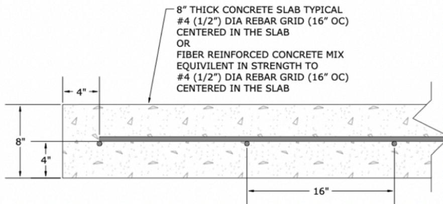
**TYPICAL 8" CONCRETE SLAB DETAIL (NOT TO SCALE)**
